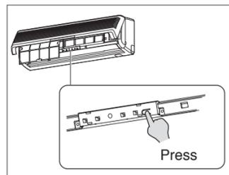
Press the MANUAL AUTO button on the main unit control panel.
