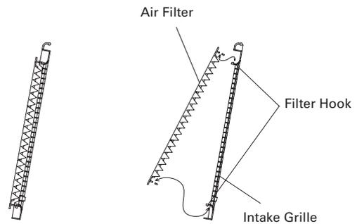
5. Close the intake grille and push the intake grille's hooks outward.
