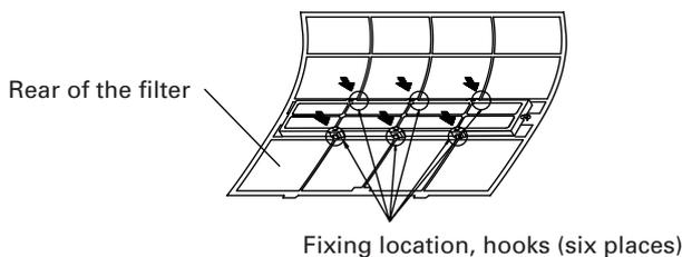
3. Install the two air filters and close the intake grille.
