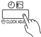
Press the timer mode button to select the ON timer or OFF timer.
