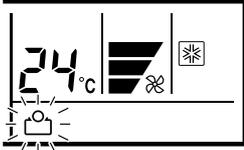
Press the ENERGY SAVE button to start or stop the energy-saving air conditioner operation.
