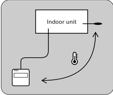
Press the THERMO SENSOR button to select whether the room temperature is detected at the indoor unit (remote sensor) or the remote controller.
