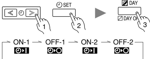
Press the set time buttons to set the time, and then press the SET button to confirm the setting and proceed to the next ON or OFF time setting. Up to two ON and OFF times can be set per day. Press the DAY button to complete the time setting and return to the day of the week setting.
