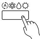
Press the master control button to set the operation mode. If DRY is selected, the fan speed will be set to AUTO.
