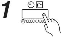
**1** Press the timer mode (CLOCK ADJUST) button for 2 seconds or more. The time display on the remote controller will flash.
