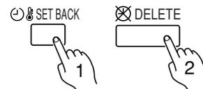
Press the SET BACK button, and then press the DELETE button while the SET BACK confirmation display is displayed. Even if the SET BACK button is pressed again, the SET BACK timer will be cancelled.
