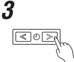
**3** Press the set time buttons to set the current time. Press repeatedly to adjust the current time in 1-minute increments. Press and hold to adjust the current time in 10-minute increments.
