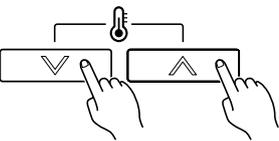
Press the set temperature buttons  $\wedge/\vee$  simultaneously for 5 seconds or more to start the self-diagnosis.
