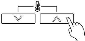
Press the set temperature buttons to set the temperature. (The temperature setting range is the same as the range for the operation mode.)
