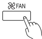
Press the FAN button to set the fan speed.
