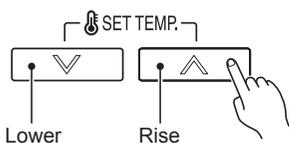
Press the SET TEMP. buttons to set the room temperature.
