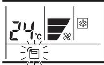
Press the ECONOMY button for more than 2 seconds to select whether the room temperature is detected at the indoor unit or the remote controller.
