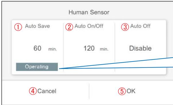
After human is not detected and the set time has passed, when "Auto Save" operation or "Auto On/Off" operation starts actually, "Operating" is displayed at "Auto Save" or "Auto On/Off".
