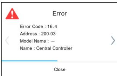
When the [Error] button is tapped, the error information (Error message or Refrigerant leakage) is displayed on the screen. Contact the service department as necessary.
