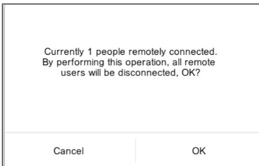
\* When some users operate remotely, the left message is displayed. When the [OK] button is tapped, all connections will be disconnected by this operation.
