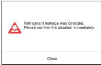
When refrigerant leakage is detected, the following message is displayed at the forefront of the screen. Confirm the error location.
