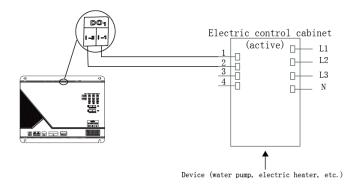
(2)The connection between the Controller DO port and the device adopts the passive electric control cabinet as shown (Only applicable for commercial water heater) :
