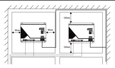
**Warning!** Power cord and communication wire of Intelligent Remote Controller must be arranged separately (with the distance over 15cm), otherwise it may cause communication error of Intelligent Remote Controller!
