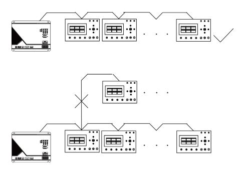
(3)Communication connection between Intelligent Remote Controller with U-Match and rooftop unit (255 sets of U-Match or rooftop unit can be connected at most).
