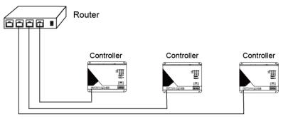
(2)Communication connection between Intelligent Remote Controller and wired controller of water heater (one Intelligent Remote Controller can connect to 16 wired controllers of water heaters at most).
