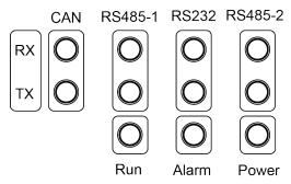
The LED indicators shown above are mainly divided into two parts: status indicators (operation, alarm, power) and communication indicators (CAN, RS485, RS2332). The following chart shows the working status of the indicators.
