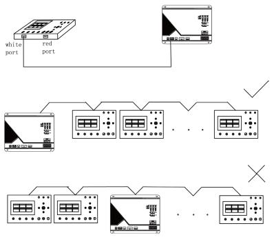
4) Communication wire connection between Intelligent Remote Controller
