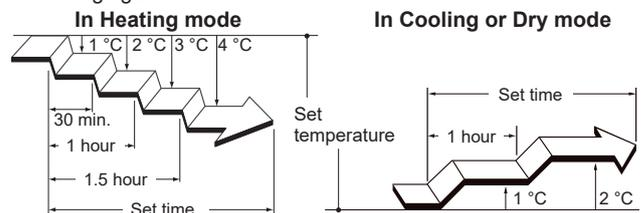
After the set time has elapsed, the air conditioner operation turns off.
